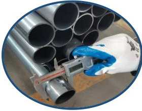
Tube Diameter Inspection
