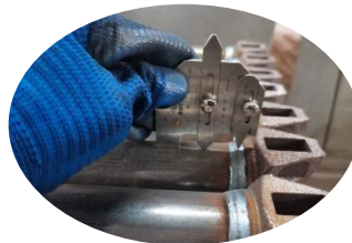
Weld Depth Inspection
